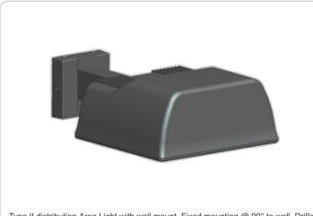
Type II distribution Area Light with wall mount. Fixed mounting @ 90° to wall. Drilling 2" on center. Factory wired for 277V. Lamp supplied.
