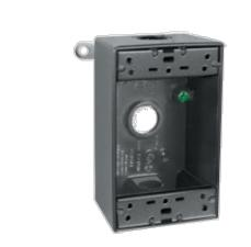
Die cast aluminum with two unique "flex-lugs" for wall or pole mounting of outdoor outlets, switches or floodlights. Ground screw and close-up plugs provided. Cubic capacity is 18.3 cu. inches.
