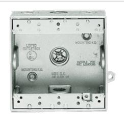
Die cast aluminum with two unique "flex-lugs" for wall or pole mounting of outdoor outlets, switches or floodlights. Ground screw and close-up plugs provided. Cubic capacity is 30.5 cu. inches.
