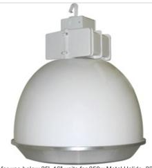
Indoor fixtures for use below 25'. 16" units for 250w Metal Halide. 22" units for 400w Metal Halide. Die cast aluminum housing, wiring box and semi specular anodized aluminum refractor. Ballast and lamp supplied.
