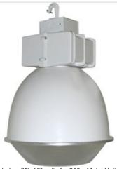
Indoor fixtures for use below 25'. 16" units for 250w Metal Halide. 22" units for 400w Metal Halide. Die cast aluminum housing, wiring box and semi specular anodized aluminum refractor. Ballast and lamp supplied.
