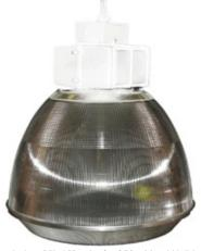
Indoor fixtures for use below 25'. 16" units for 250w Metal Halide. 22" units for 400w Metal Halide. Die cast aluminum housing and wiring box. Clear acrylic Lexalite Reflexor prismatic refractor. Ballast and lamp supplied.
