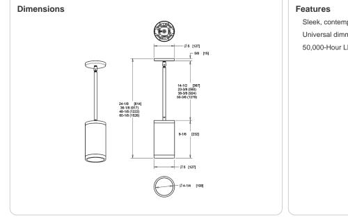
Sleek, contemporary, architectural-grade design Universal dimming driver (TRIAC, ELV and 0-10V) 50,000-Hour LED lifespan
