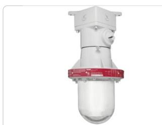
Explosionproof fixture for ceiling mounting. Cast aluminum housing, heat and impact resistant globe. Fits all incandescent lamps up to 300 Watt PS-25. Lamp not supplied.
