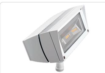
Rectangular shaped LED floodlight designed to replace 70W Metal Halide. Patent Pending airflow technology ensures long LED and driver lifespan. Use for building facade lighting, sign lighting, LED landscape lighting and instant-on security lighting. Weight: 4.8 lbs
