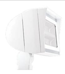
Ultra high output, high efficiency LED floodlight with twistlock photocell. Available with wide NEMA type 6H x 6V beam spread. Patent Pending airflow technology ensures long LED and driver lifespan. Use for general and security lighting for large areas, building facades, signs and landscapes.
