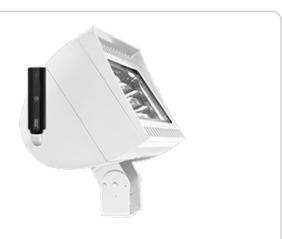
Ultra high output, high efficiency LED floodlight with NEMA Types: 7H x 6V, 6H x 4V, 4H x 6V, 5H x 5V and 3H x 3V. Patent Pending airflow technology ensures long LED and driver lifespan. Use for general and security lighting for large areas, building facades, signs and landscapes. Includes built in support for Lightcloud, a wireless lighting control system and service, fully developed by RAB.
