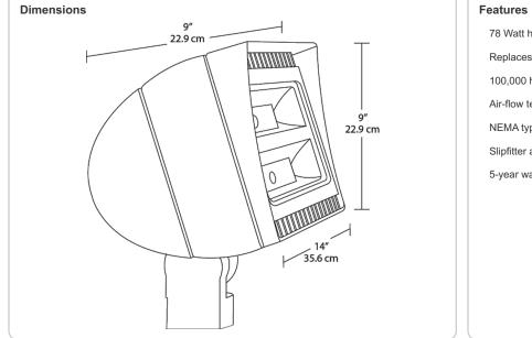
78 Watt high-performance LED Replaces 250W MH floodlights 100,000 hour life based on LM-80 tests Air-flow technology heatsink NEMA type - 6H x 6V Slipfitter and trunnion mounting available 5-year warranty
