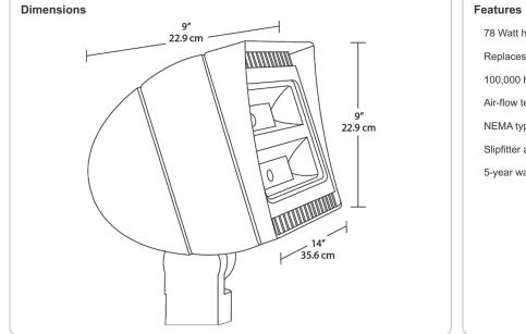
78 Watt high-performance LED Replaces 250W MH floodlights 100,000 hour life based on LM-80 tests Air-flow technology heatsink NEMA type - 6H x 6V Slipfitter and trunnion mounting available
