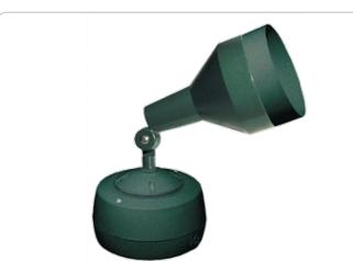
Large size flood for easier relamping and glare reduction. Durable one piece die casting with rugged mounting arm, weatherproof gasket and drain holes. Accepts 150 Watt PAR 38 max. Lamp not supplied.
