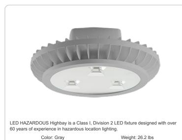
Project: Type: Prepared By: Date: **Driver Info** LED Info Type: Constant Current Watts: 78W 120V: 0.82A Color Temp: 5000K 208V: 68 CRI 0.52A Color Accuracy: 240V: 0.45A 100000 L70 Lifespan: 277V: 0.4A Lumens: 6,322 Input Watts: 96W Efficacy: 66 LPW Efficiency: 81%
