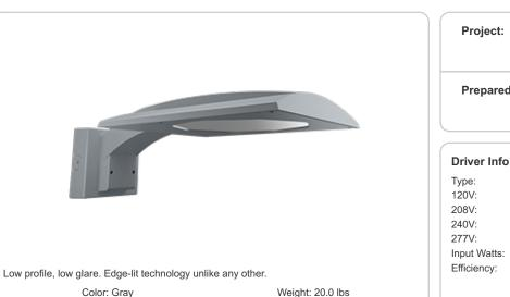
Type: **Prepared By:** Date: LED Info Constant Current 67W Watts: 0.58A Color Temp: 5000K (Cool) 0.34A Color Accuracy: 74 CRI 0.29A L70 Lifespan: 100,000 0.25A Lumens: 7.927 68W Efficacy: 116 LPW
