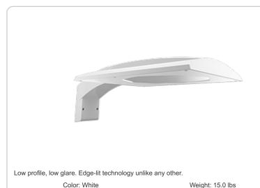
Project: Type: **Prepared By:** Date: **Driver Info** LED Info Constant Current 117W Type: Watts: 120V: 1.00A Color Temp: 4000K (Neutral) 208V: 0.58A Color Accuracy: 72 CRI 240\/-0.50A L70 Lifespan: 100,000 277V: 0.43A Lumens: 13.357 Input Watts: 115W Efficacy: 116 LPW Efficiency: N/A
