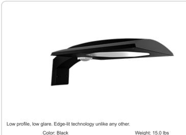
Prepared By: Date: **Driver Info** LED Info Constant Current 38W Type: Watts: 120V: N/A Color Temp: 4000K (Neutral) 208V: N/A Color Accuracy: 72 CRI 240\/-N/A L70 Lifespan: 100,000 277V: N/A 5.530 Lumens: Input Watts: 43W Efficacy: 130 LPW
