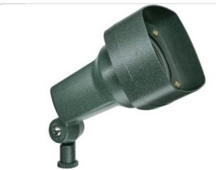
Rugged die cast floodlight with heavy mounting arm, lens, glare shield and weatherproof silicone gasket. 75 Watt max., accepts lamp types PAR16, PAR20 and R type. 120 volt Lamp not supplied.
