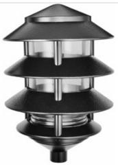
Rugged die cast aluminum 6" diameter housings. Threaded, gasketed clear glass globe for durable weatherproofing and easy relamping. 1" long, 1/2" threaded nipple included for easy mounting. 100 Watt max. Incandescent lamp not supplied. Fluorescent lamp supplied.
