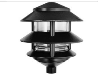
Rugged die cast aluminum 6" diameter housings. Threaded, gasketed clear glass globe for durable weatherproofing and easy relamping. 1" long, 1/2" threaded nipple included for easy mounting. 75 Watt max. Incandescent lamp not supplied. Fluorescent lamp supplied.
