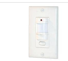
Fits decorator wall plates with only 1/2" protrusion. 120 volts. Gangable. Full 180° view covers 1000 sq. ft Works with electronic ballasts. Can be wired in parallel. LED indicator, wallplate included. Can also be used as a ceiling sensor. Must have hot and wires in box.
