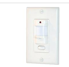
Fits decorator wall plates with only 1/2" protrusion. 120 volts. Gangable. Full 180° view covers 1000 sq. ft Works with electronic ballasts. Can be wired in parallel. LED indicator, wallplate included. Can also be used as a ceiling sensor. Must have hot and wires in box.
