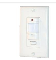
Meets California Title 24 standards. Must be turned on manually, but shuts off automatically. Full 180° view covers 1000 sq. ft. Works with electronic ballasts. Can be wired in parallel. LED indicator, wallplate supplied. Can also be used as a ceiling sensor. Must have hot, common & ground wires in box.
