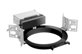
Easy to install 6" rough-in with die-cast aperture ring, removable driver, thermal protector and adjustable butterfly brackets. This rough-in is designed to make new construction recessed downlighting easy Available with 80 or
