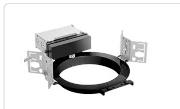
Easy to install 6" rough-in with die-cast aperture ring, removable driver, thermal protector and adjustable butterfly brackets. This rough-in is designed to make new construction recessed downlighting easy Available with 80 or
