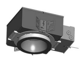
Easy to install 6" rough-in with die-cast aperture ring, removable driver, thermal protector and adjustable butterfly brackets. This rough-in is designed to make new construction recessed downlighting easy Available with 80 or
