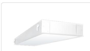
1' x 4' LED panel lights with emergency battery Backup that will operate the LED Lamp for 90 minutes if power fails. For use in drop ceilings or drywall using the optional recessed mounting kit.
