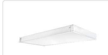
2' x 4' LED panel lights with emergency battery Backup that will operate the LED Lamp for 90 minutes if power fails. For use in drop ceilings or drywall using the optional recessed mounting kit.
