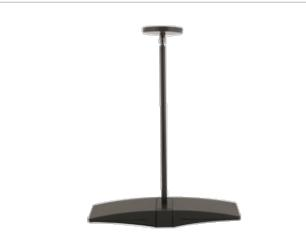
The PLED is a high performance LED downlight available in 52, 40, 26 and 20W versions in both Cool and Warm Color Temperatures. Pendant mount with hangstraight and 6", 12" and 18" stems included. Stems can be combined up to 36" max length.
