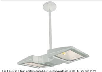
The PLED is a high performance LED uplight available in 52, 40, 26 and 20W versions in both Cool and Warm Color Temperatures. Pendant mount with hang-straight and 6", 12" and 18" stems included. Stems can be combined up to 36" max length.
