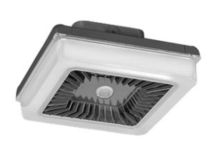
This ultra high efficiency LED large garage light delivers up to 111 lumens per Watt. An integrated motion/photo sensor option provides multi-level lighting control. Available in 70, 80 and 105W versions. Fixture measures 18" L x 18" W.
