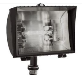
The Mini Curve. High quality die cast flood with rounded back and integral glare shield. Tempered glass lens. Gold plated socket contacts and 250°C Teflon coated wires for extended lamp life. 200 Watt double ended 130 volt Quartz halogen lamp supplied.
