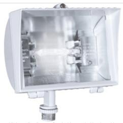
The Mini Curve. High quality die cast flood with rounded back and integral glare shield. Tempered glass lens. Gold plated socket contacts and 250°C Teflon coated wires for extended lamp life. 200 Watt double ended 130 volt Quartz halogen lamp supplied.
