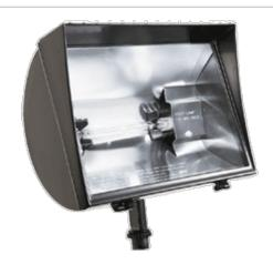
300 Watt Quartz flood with round back and cast aluminum Integra Hood. Hinged lens frame permits easy relamping. Stainless steel locking clip. Gold plated socket contacts and 250°C Teflon coated wires for extended lamp life. Lamp supplied.
