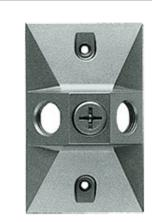
Die cast rectangular covers with one or three 1/2" threaded holes. Fits FS, cast and recessed single outlet boxes. Supplied with thick foam rubber gasket and two #6-32 stainless steel screws. 3 hole cover comes with one die cast 1/2" close-up plug.
