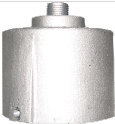
Aluminum Pole Slipfitters for mounting fixtures or boxes to top of poles or posts. 1/2" top tap standard. 3/4" top tap on R5-3/4 and R7-3/4 only. Set screws provided.
