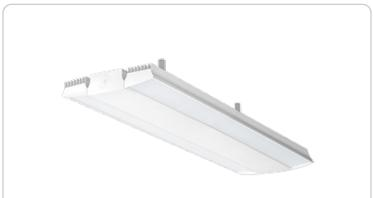
LED High Bay fixture ideal for large indoor spaces, including warehouses, gymnasiums and distribution centers with high ceiling that require mounting heights of 50-60 feet. Replaces up to 1000W MH fixtures.
