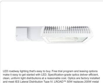
Project: Type: Prepared By: Date: **Driver Info** LED Info Type: Constant Current Watts: 50W 120V: 0.46A Color Temp: 5000K 208V: 0.27A Color Accuracy: 67 CRI 240V: 0.23A 100000 L70 Lifespan: 277V: 0.20A Lumens: 5,196 Input Watts: 52W Efficacy: 100 LPW Efficiency: 96%
