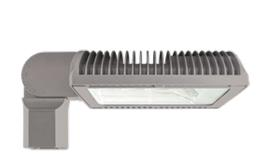
LED roadway lighting that's easy to buy. Free trial program and leasing options make it easy to get started with LED. Specification-grade optics deliver efficient, clean, uniform light distributions at a reasonable cost. Optics are factory installed and meet IES Lateral Distribution Type IV. LROAD<sup>™</sup> 78W replaces 250W metal halide roadway fixtures.
