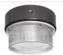
11" or 15" round fixture. 35, 50, 70, 100 & 150w HPS lamp or 50, 70 & 100 Watt Metal Halide. Housing is die formed heavy gauge aluminum in bronze enamel finish with clear vandalproof polycarbonate refractor. Lamps supplied.
