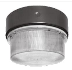
11" or 15" round fixture. 35, 50, 70, 100 & 150w HPS lamp or 50, 70 & 100 Watt Metal Halide. Housing is die formed heavy gauge aluminum in bronze enamel finish with clear vandalproof polycarbonate refractor. Lamps supplied.
