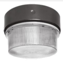
11" or 15" round fixture. 35, 50, 70, 100 & 150w HPS lamp or 50, 70 & 100 Watt Metal Halide. Housing is die formed heavy gauge aluminum in bronze enamel finish with clear vandalproof polycarbonate refractor. Lamps supplied.
