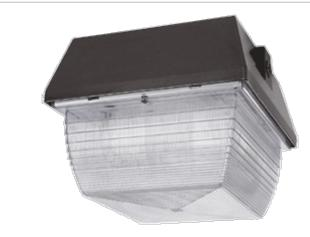
Medium size ceiling mount fixture: 26, 32 and 42 Watt compact fluorescent available. Housing is die cast aluminum with clear vandalproof polycarbonate refractor. Photocontrol, Sensor (CFL 120v only) models available. Lamp supplied.
