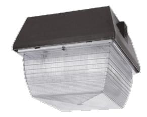
Medium size ceiling mount fixture: 35, 50 and 70 Watt HPS, 50 and 70 Watt Metal Halide. Housing is die cast aluminum with clear vandalproof polycarbonate refractor. Quartz Restrike models available. Lamps supplied.
