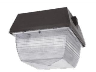
Medium size ceiling mount fixture: 35, 50 and 70 Watt HPS, 50 and 70 Watt Metal Halide. Housing is die cast aluminum with clear vandalproof polycarbonate refractor. Quartz Restrike models available. Lamps supplied.
