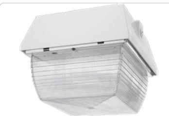
Medium size ceiling mount fixture: 35, 50 and 70 Watt HPS, 50 and 70 Watt Metal Halide. Housing is die cast aluminum with clear vandalproof polycarbonate refractor. Quartz Restrike models available. Lamps supplied.
