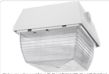
Medium size ceiling mount fixture: 35, 50 and 70 Watt HPS, 50 and 70 Watt Metal Halide. Housing is die cast aluminum with clear vandalproof polycarbonate refractor. Quartz Restrike models available. Lamps supplied.
