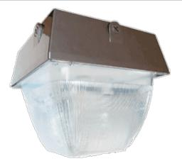
VAN5 12" x 12" Emergency Battery Backup. 2x 32W CFL or 2x 42W CFL. Available in 120V or 277 volts. Emergency battery operates only one lamp. Lamp supplied.
