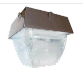
Large size ceiling mount fixture. Vertical lamp HID. Adjustable, 4-way glare guard & "No Bend" conduit entrance. Excellent heat control eliminates heat problems. Housing is die cast aluminum with clear vandalproof polycarbonate refractor. Lamps supplied.
